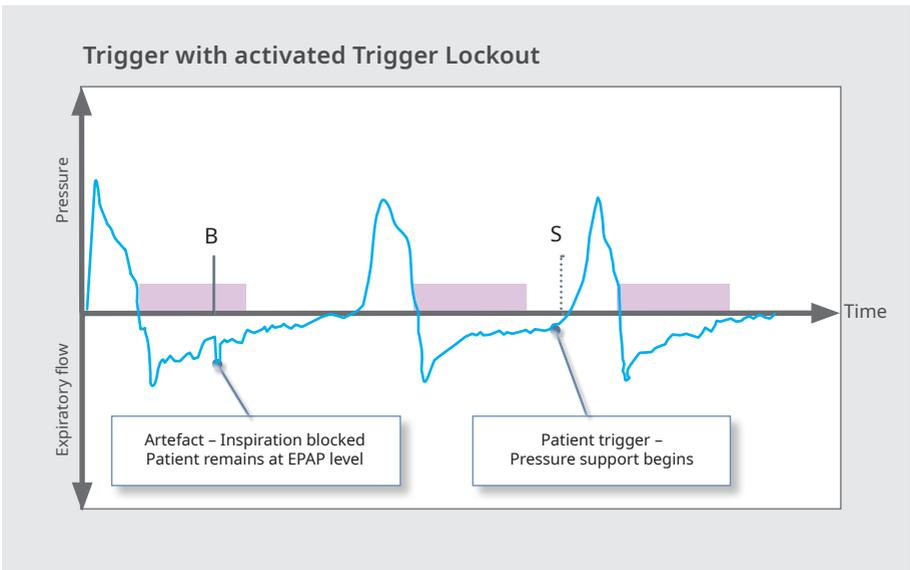
Figure 29 The setting of a suitable Trigger Lockout period prevents the ventilator from making a premature switch to inspiratory phase (see Figure 28).
