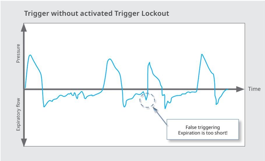
Figure 28 Assisted ventilation with false triggering caused by fluctuations in the flow curve with a sensitively set trigger without Trigger Lockout.
